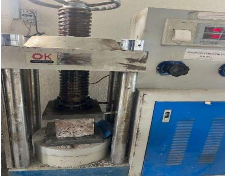
Figure 10: Compressive strength test on concrete cubes
