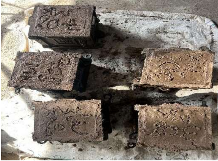
Figure 9: Cast geopolymer concrete
